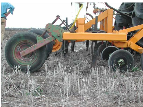
**Figure 20.** Modified anhydrous ammonia rig with coulters discs in front of gas knives
